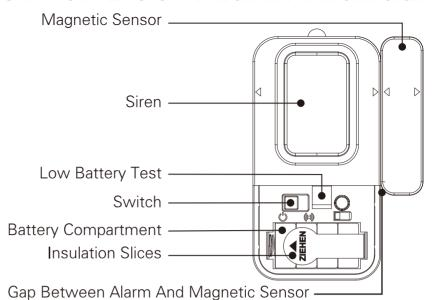
(Alarm is activated when switched ON and gap between alarm and magnetic sensor is greater than 1/2")
