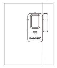
**Step 3:** Open battery cover, remove battery insulating trio and push switch to ON position, then close battery cover.
