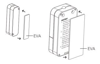
Step 2: Placing one of the units on the part of the fixture that opens (window) and the other unit on the stationary part of the fixture (frame). Mount so that when the window, door or cabinet is closed, the gap between the alarm and sensor is no more than 1/2" (preferably less).
